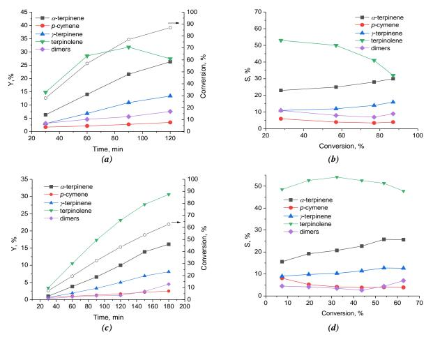
Figure 7. Conversion, product yields (*a*, *c*) *vs*. reaction time, and selectivity *vs*. conversion (*b*, *d*) on the samples K2 (*a*, *b*) and K1 (*c*, *d*).
