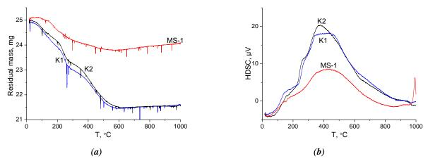
Figure 8. TG (a) and DTA (b) curves of MS-1, K1, and K2 deactivated samples.
