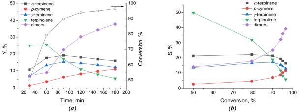
Figure 6. Conversion, product yields vs. reaction time (a), and selectivity vs. conversion (b) on the sample MS-1.
