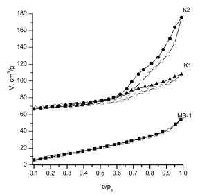
Figure 2. Isotherms of low-temperature nitrogen adsorption for a number of samples from kaolin.
