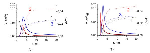
Figure 3. Integral and differential pore size distributions calculated from BJH theory using the adsorption (*a*) and desorption (*b*) branches of isotherms for MS-1 (*I*), K1 (*2*), and K2 (*3*).
