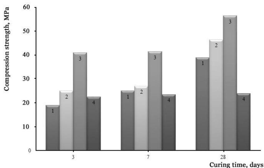
**Figure 3. A histogram illustrating the increase in compressive strength of various formulations of construction binders mixed with combustion ash: PC400 - 1; PC500 - 2; 75%PC400+25%CC - 3; 50%PC400+50%CC - 4. (where, PC – Portland cement, CC – CAS ash)**
