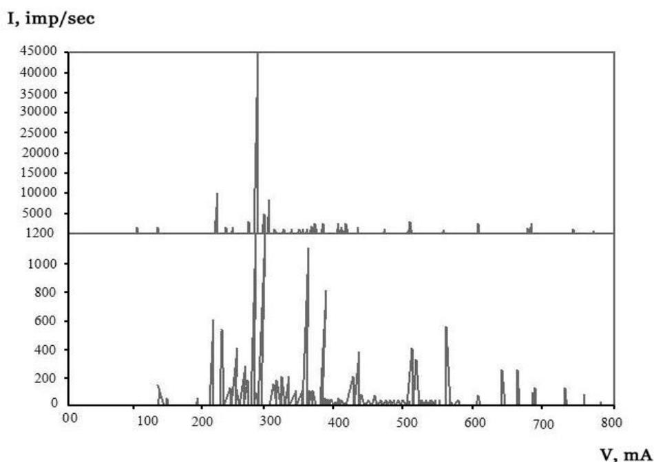
**Figure 2. The X-ray diffraction data collected for CAS ash.**
