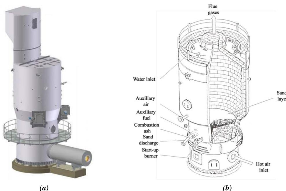
Figure 1. Representation of the “Pyrofluid” furnace (a) and its sectional schematic view (b).
