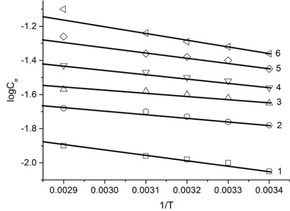
**Figure 6.** Isotherms of strontium ion adsorption from aqueous solutions on activated carbon CAN-8, at specific adsorption values: (1)- 0.025 mmol/g, (2)- 0.05 mmol/g, (3)- 0.075 mmol/g, (4)- 0.1 mmol/g, (5)- 0.125 mmol/g, (6)- 0.15 mmol/g.
