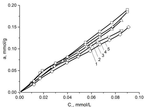
**Figure 3.** Adsorption isotherms of strontium ions from aqueous solutions on activated carbon CAN-7, at different temperatures: (1)- 25°C, (2)- 35°C, (3)- 45°C, (4)- 55°C, (5)- 65°C.
