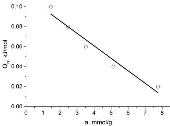
**Figure 7.** Correlation of the adsorption isosteric heat ( $Q_{is}$ ) of strontium ions on the activated carbon CAN-7 and the specific adsorption  $a$ .
