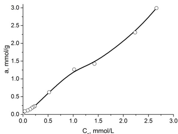
Figure 1. Adsorption isotherm of strontium ions from aqueous solutions on the activated carbon CAN-7.
