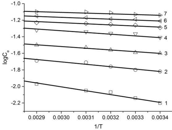
**Figure 5.** Isotherms of strontium ion adsorption from aqueous solutions on activated carbon CAN-7, at specific adsorption values: (1)- 0.02 mmol/g, (2)- 0.04 mmol/g, (3)- 0.06 mmol/g, (4)- 0.08 mmol/g, (5)- 0.1 mmol/g, (6)- 0.12 mmol/g, (7)- 0.14 mmol/g.
