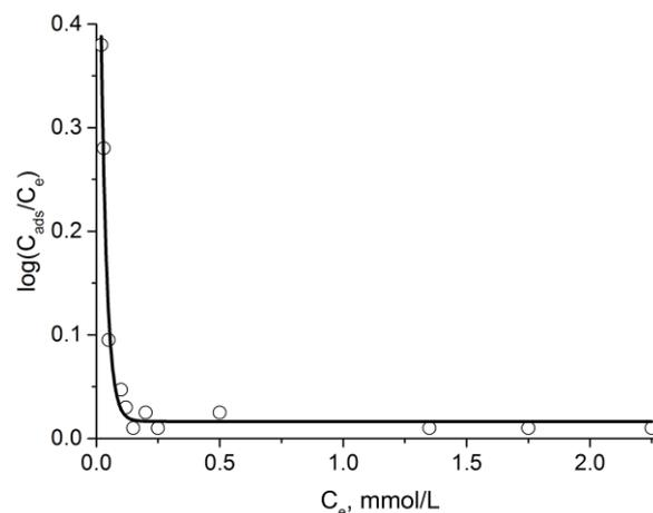
Figure 2. The isotherm of adsorption of strontium ions from aqueous solutions on the activated carbon CAN-7, in the coordinates of  $\log(C_{ads}/C_e)$  vs.  $C_e$ , at  $t = 25^\circ\text{C}$ .
