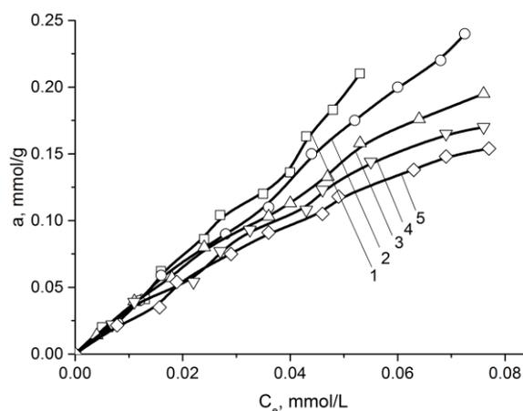
**Figure 4.** Adsorption isotherms of strontium ions from aqueous solutions on the activated carbon CAN-8, at different temperatures: (1)- 25°C, (2)- 35°C, (3)- 45°C, (4)- 55°C, (5)- 65°C.
