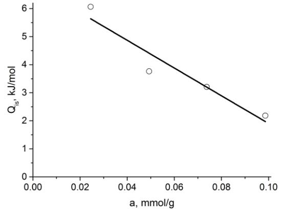
**Figure 8.** Correlation of the adsorption isosteric heat ( $Q_{is}$ ) of strontium ions on the activated carbon CAN-8 and the specific adsorption  $a$ .
