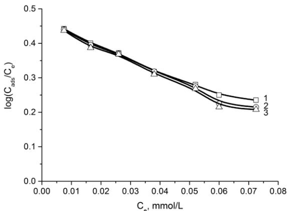
**Figure 9.** Adsorption isotherms of strontium ions from aqueous solutions on the activated carbon CAN-7 in the coordinates of  $\log(C_{ads}/C_e)$  vs.  $C_e$ , at (1)- 35°C, (2)- 45°C and (3)- 55°C.
