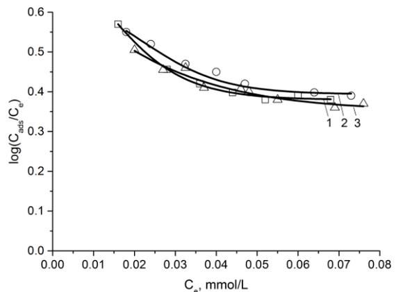
**Figure 10.** Adsorption isotherms of strontium ions from aqueous solutions on activated carbon CAN-8 in the coordinates of  $\log(C_{ads}/C_e)$  vs.  $C_e$ , at (1)- 35°C, (2)- 45°C and (3)- 55°C.
