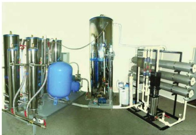
**Fig.3. Multifunctional module installation “Vega-3UM” with productivity of 5000 liters per hour**
