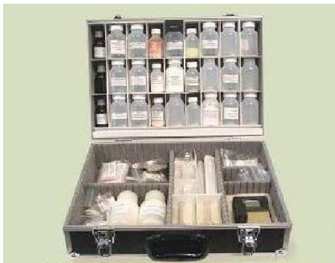
**Fig. 4. Portable laboratory "Aqua-test" for monitoring water quality.**
