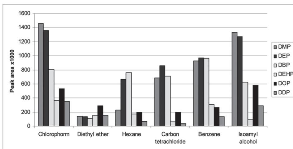
Fig. 1. Signals intensity of phthalates in various extractants
