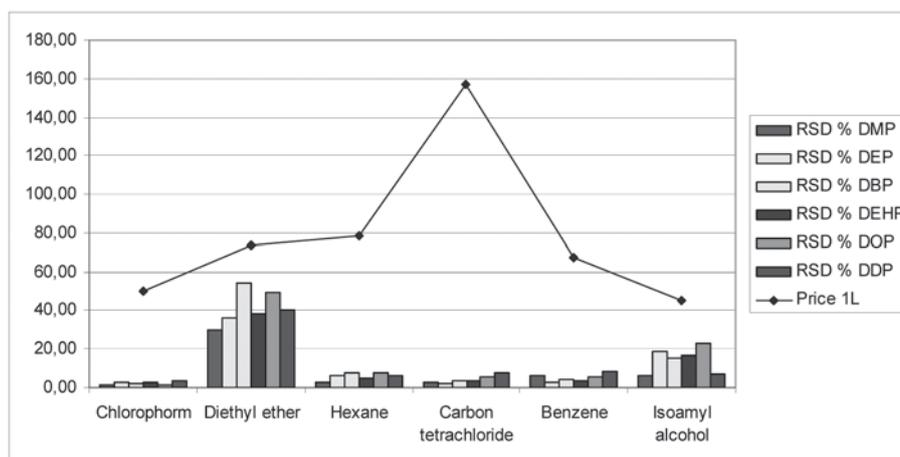
**Fig. 2.** Relative standard deviation of four extractions. Prices of organic solvents for 1L/€\*
