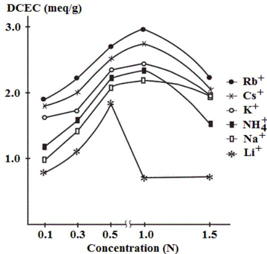
Figure 4. Dynamic ion exchange capacity of Georgian scolecite for monovalent cations at different concentration of solutions.
