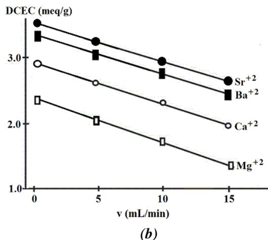
Figure 5. Dynamic ion exchange capacity of Georgian scolecite for monovalent (a) and bivalent (b) cations at different flow rates.
