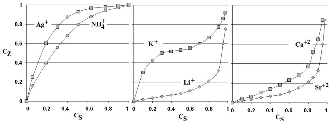
Figure 1. Ion exchange isotherms on analcime.
