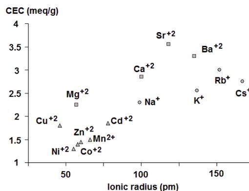
Figure 3. Exchange capacity versus ionic radius.
