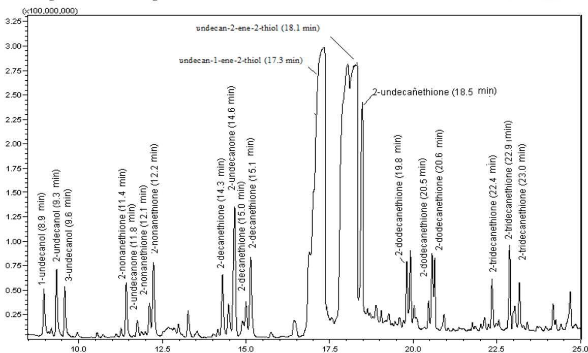
Figure 3. Chromatogram of thionated essential oils from *Ruta montana* L. (S-EO<sub>RM</sub>).
